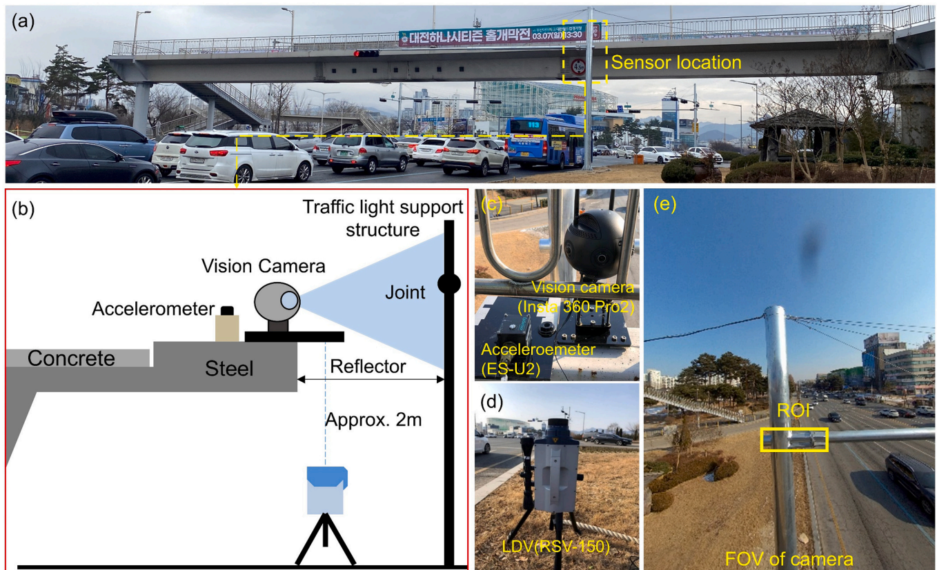
Fig. 15. Configuration of pedestrian steel box-girder bridge test: (a) overview of the bridge, (b) sensor setup, (c) an accelerometer and a vision camera used for displacement estimation, (d) an LDV for reference displacement measurement, and (e) FOV of camera and the initial ROI.
